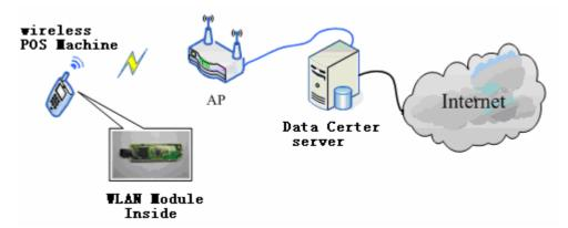
In a Wireless Bus System based on the WLAN technique, carheld or handheld POS machine in each bus equips with a WIFI module, and AP is fixed in the Bus Terminus. When buses reach the terminus, wireless POS machine always does the identification automatically, then connect to the AP, and Operational Data in POS machines is uploaded to Data Center Server in Bus Terminus through AP.
